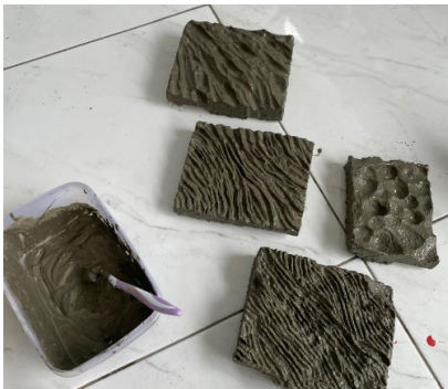
Figure 8: Experimental modules testing the adhesion and structural integrity of cementitious coatings on varied textures. (Photo: Caraka Aji PJ, 2024)
