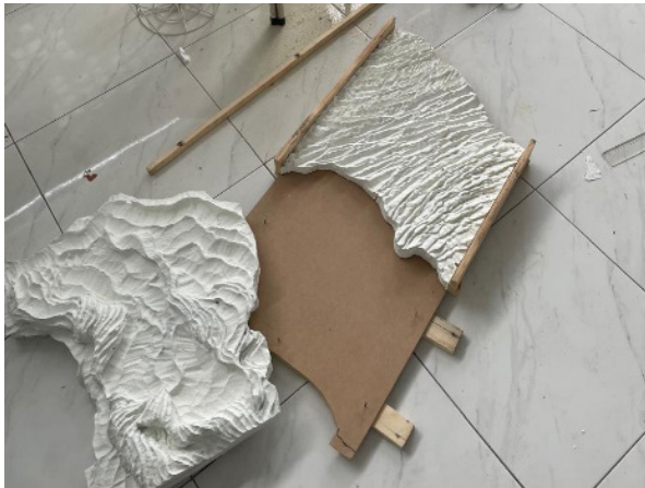
Figure 9: Preparation of the structural frame and finalization of carved modules prior to composite application. (Photo: Caraka Aji PJ, 2024)
