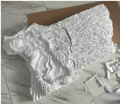
Figure 7: Visual comparison between raw EPS surface and the sinuous textures achieved through carving and thermal application. (Photo: Caraka Aji PJ, 2024)
