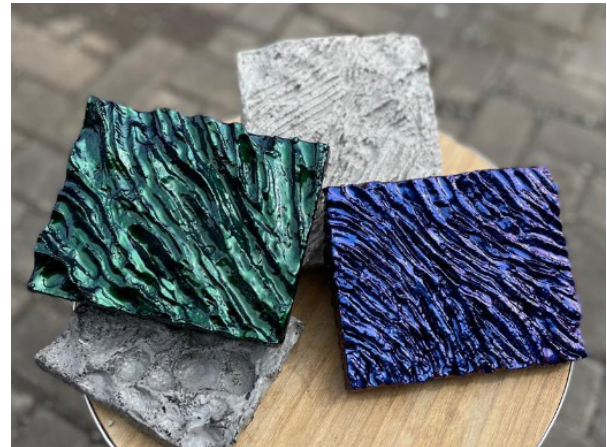
Figure 10: Polychromatic color testing on cement-coated modules to determine optimal light reflection and color depth. (Photo: Caraka Aji PJ, 2024)
